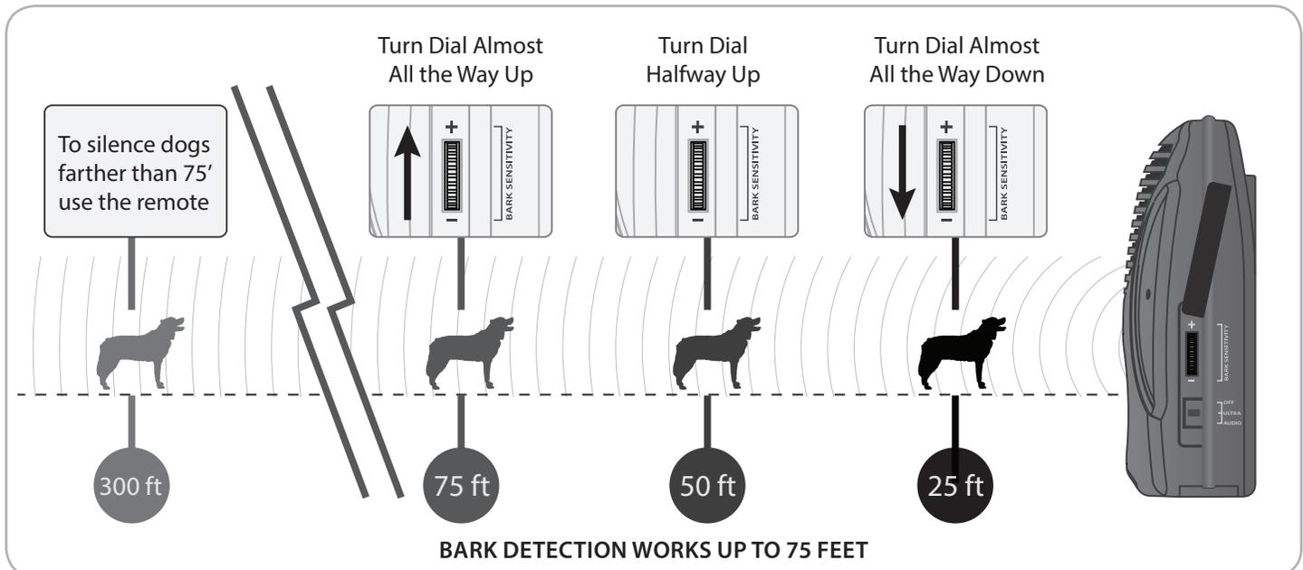
3 Slide the Power Switch to 'Audio' while configuring the Bark Sensitivity Dial. This way, you can hear when the Dog Silencer MAX activates and adjust the sensitivity accordingly. Audio also works great for dogs with some hearing loss. **IMPORTANT: The Bark Sensitivity Dial is not a volume dial. The volume on the Dog Silencer is always set to the maximum and is not adjustable.**
